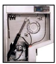
Hydraulic Tilt Mechanism Side With Special Operator Controls
